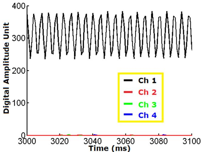
Fig. 4. Time domain plots. The sine wave (223 Hz) was only sent to Channel 1.
